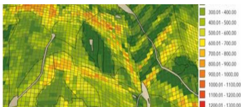
Figure 54 Tridimensional visualization of CHM-predicted forest stand attributes (grid cell 20 x 20 m) (source: Sačkov, 2022)
